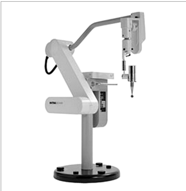
Fig 1. Intrabeam™ system ①Robotic arm ②50kVp X-ray Source(XRS) ③Spherical applicator
