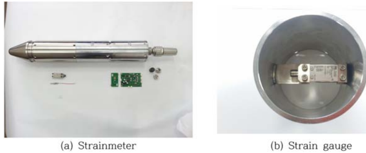
Fig. 1. Strainmeter installed around the Andong fault zone.
