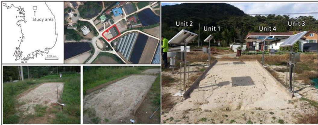
Fig. 1. Test bed for monitoring soil erosion.
