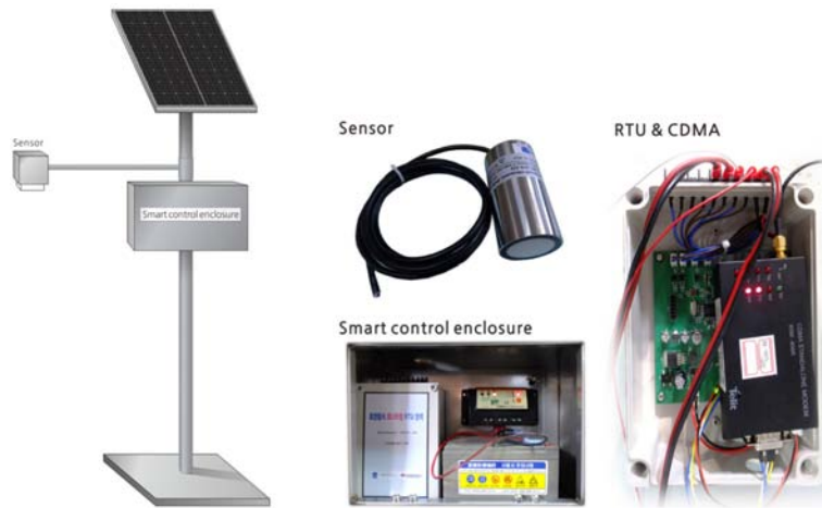
Fig. 3. Schematic figure and photographs of the soil-erosion monitoring device.
