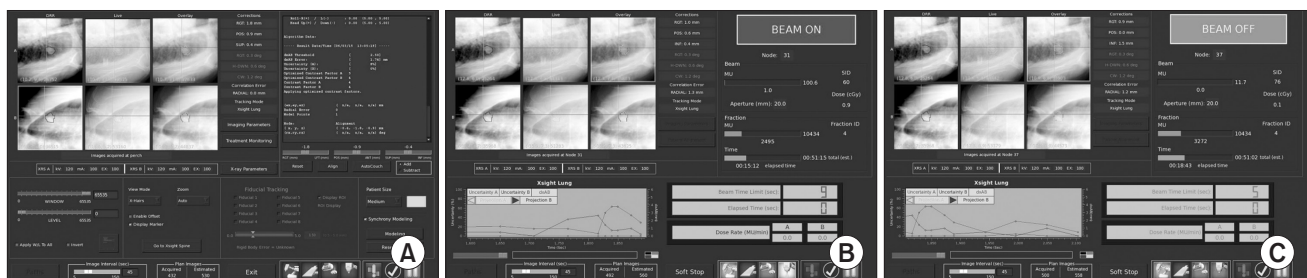
Fig. 1. Xsight lung tracking system. (A) Tracking. Before radiation delivery, Xsight lung tracking system starts to track the tumor. It will take about 5–10 minutes. (B) Beam on. If Xsight lung tracking system localized the tumor, delivery of radiation starts. (C) Beam off. If Xsight lung tracking system missed the tumor, delivery of radiation stops and the system re-tracks the location of tumor.
