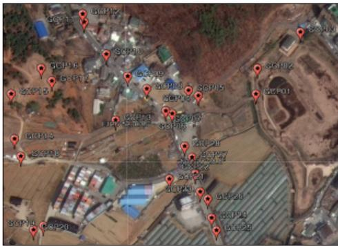
Figure 7. Ground control point
