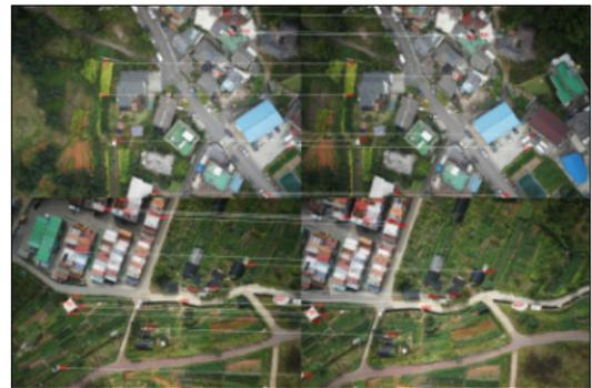
Figure 9. Extracted tie-points
