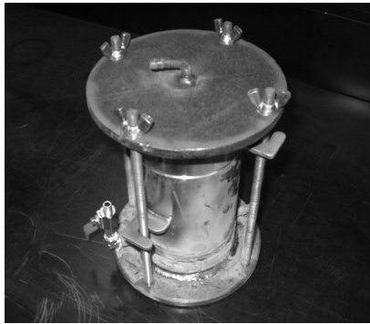
Fig. 4. Modified mold of permeability test
