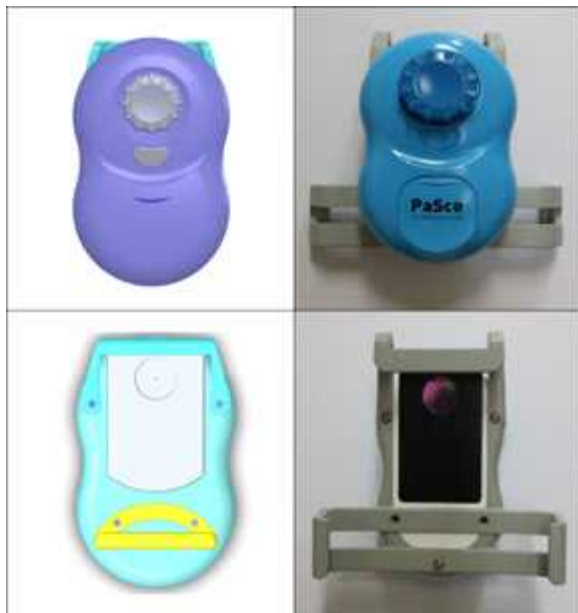
Fig. 2 3D model (left) and prototype (right) of an optical adaptor for fluorescence smartscope
