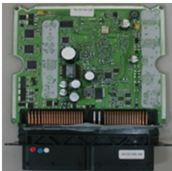
Fig. 1 Photograph of electronic control module soldered with SAC305 for engine control
