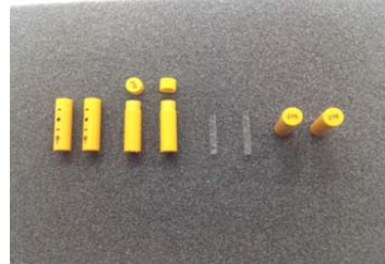
Fig. 2. Glass dosimeter used for patient dose measurement.
