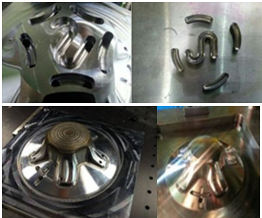
Fig. 9 Hybrid cladding process of wheel hubcap
