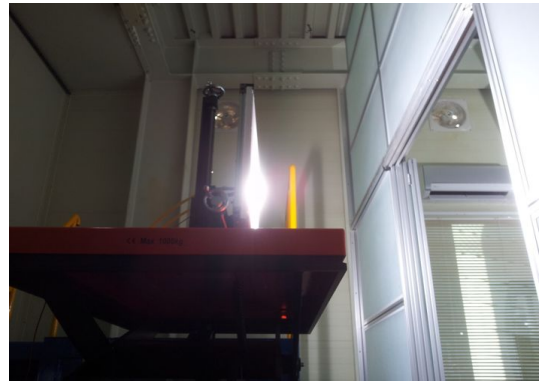
Fig. 3 Light concentrated on the diffuse target surface during flux measurement
