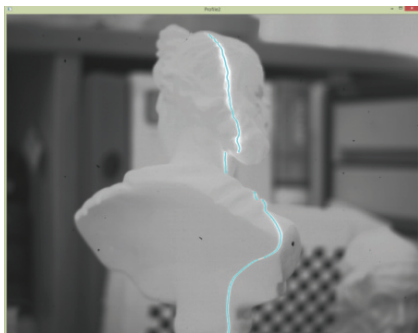
Fig. 12 Laser profile extracted from additional camera
