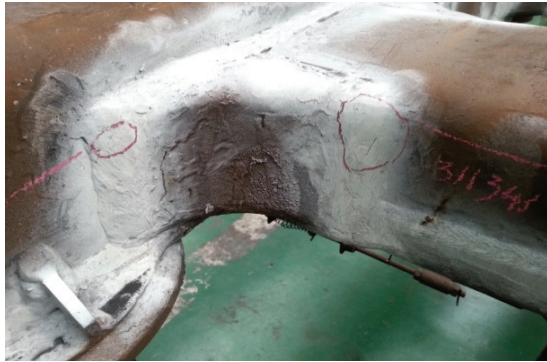
Fig. 1 Fatigue crack in bogie frame
