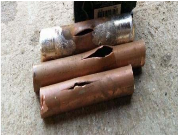
Fig. 4 Pipe bursting due to excessive internal pressure
