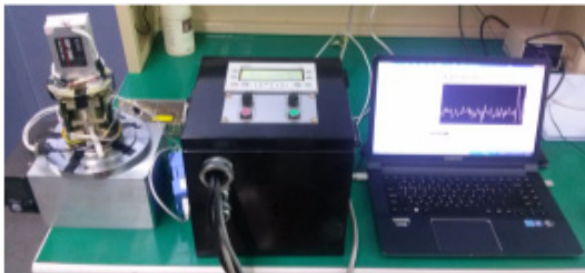
Fig. 4 Gyroscope characteristic verification Test Equipment system
