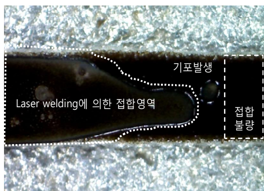
Fig. 5. Observation of glass welding section laser welded
