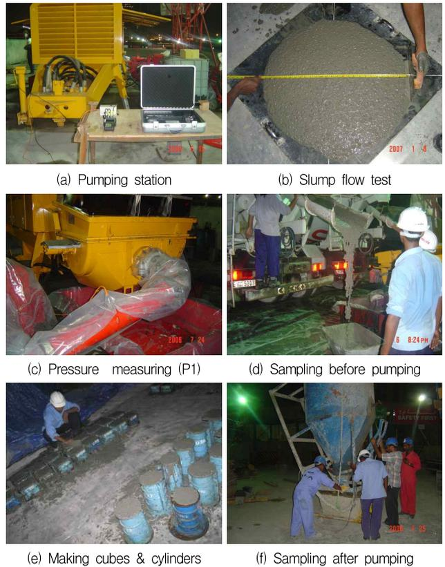
Figure 6. Pressure measuring and concrete testing
