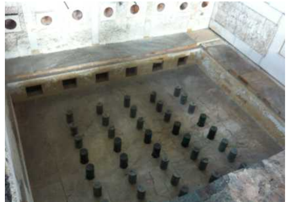
Figure 3. Specimen preparation for fire-resistance test
