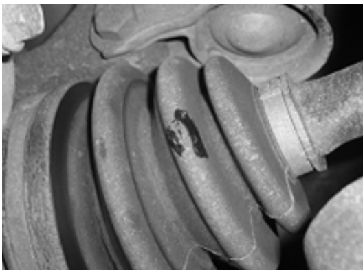
Fig. 6. Grease leaking example of drive shaft boots.
