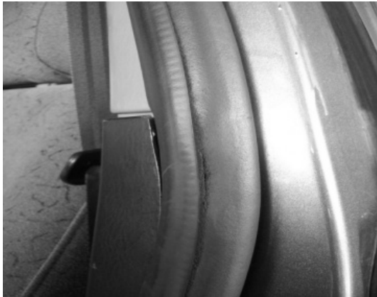
Fig. 8. Tearing example of door weather strip molding.
