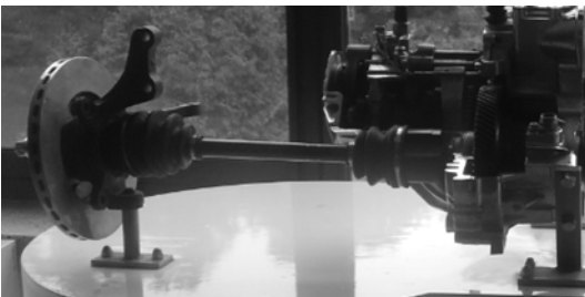
Fig. 2. Assembling example of C.V joint boots.
