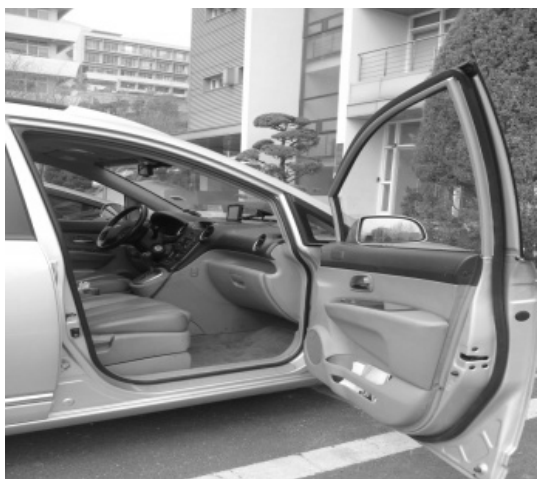
Fig. 7. Weather strip installing example in door around and body contacting part of a car.
