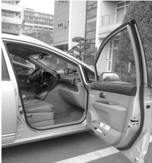
Fig. 3. Door weather strip inserted inside door.
