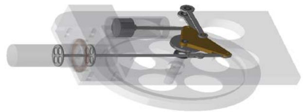
Figure 14: Designed \gamma -type Ross yoke driver Stirling engine
