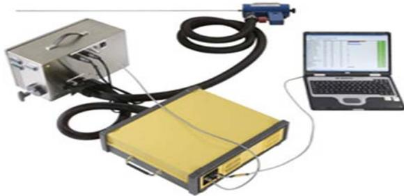
Figure 7: FTIR method measurement equipment
