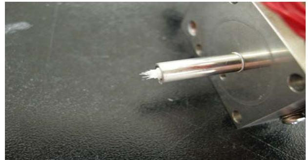
**Figure 11:** White precipitate was produced in NO<sub>x</sub> conversion unit
