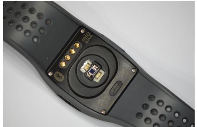
Fig. 2. Back face of Mio Alpha shows light emitting diode sensors.
