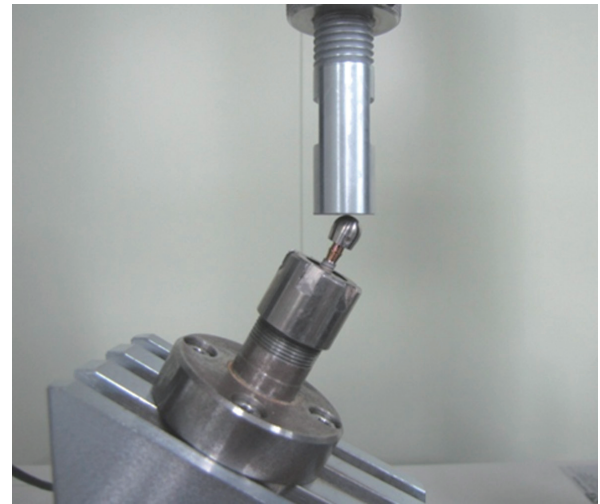
Fig. 2. Photograph depicting the installation of Ti implants and abutment complex for the static compressive strength test. The axis of the loading direction against the axis of the dental implant system was 30°.
