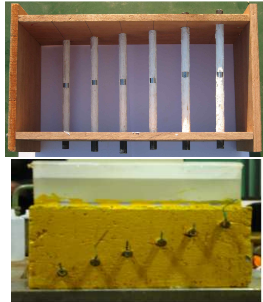
Fig. 1. Photo. of (a) mold box for conducting multiple test specimen and (b) molded multiple specimens for multiple test.
