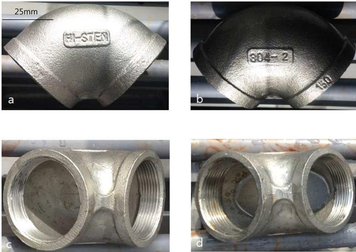
Fig. 6. Result of 2-hr salt spray test of (a) and (c) heat treated specimen and (b) and (d) non-heat treated specimen.
