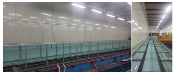
Fig. 2. Supercavitation water tank (KAIST)
