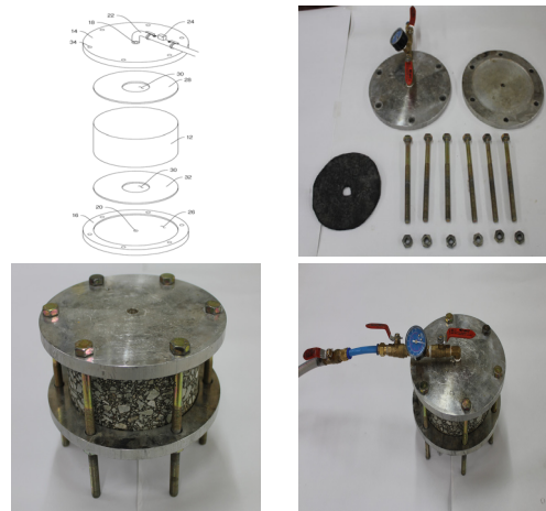
[Fig. 5] permeability measuring device
