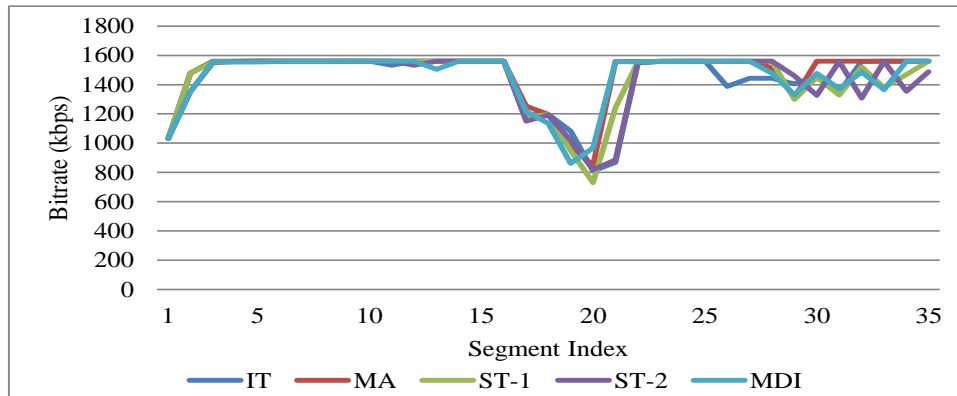
Fig. 2(a). Throughput observed by the client based on the implementation of each throughput estimation method
