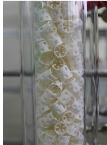
Fig. 4 Column packed with Pall rings produced in this study.
