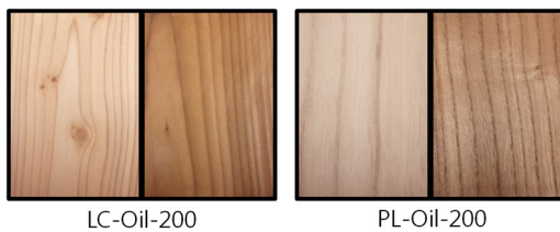
Fig. 8. Photos of the control and oil heated larch and paulowniawood specimens, taken at 4mm below the surfaces.
