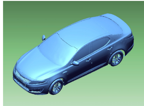
Fig. 5 K5(2011) mesh model using 3D scanner
