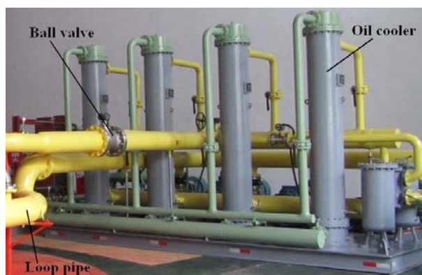
Fig.1. The lubricating and cooling pipe systems of test-bed
