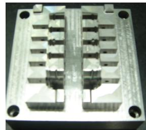
Fig. 13 (a) core particles by DMLS & NC integrated machines
