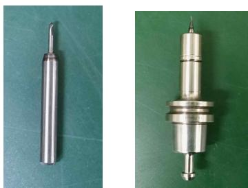
Fig. 4 (a) NC Tool (b) tool holder
