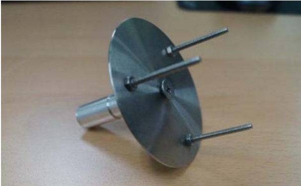
Fig. 5 A tripod jig pushing an ice down in the water
