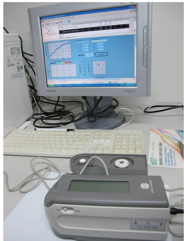
Fig. 2. Spectrophotometric analysis. The machine for spectrophotometric analysis (CM-2600d) and CIE L*a*b* software are shown.
