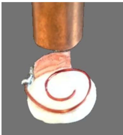
Fig. 3. The fabricated prototype of the spiral monopole antenna. The connected coaxial cable and balun are seen at the top.
