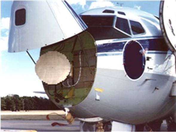
Fig. 11. Aircraft, weather radar antenna (transmit-array) under a radome (frequency selective surface).
