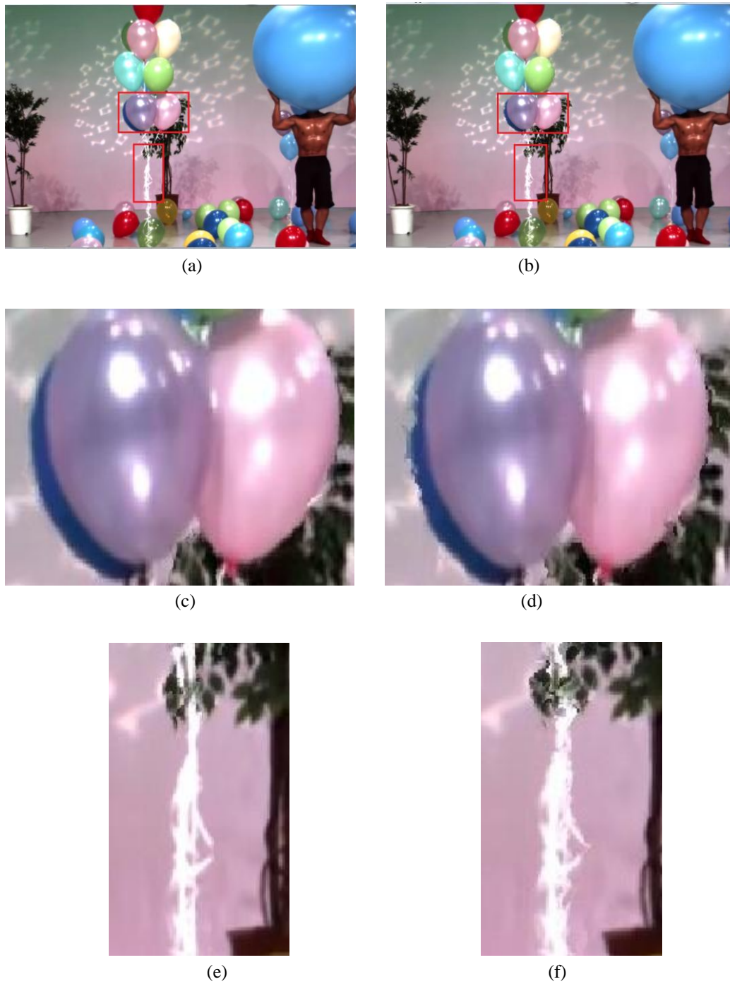
Fig. 7. Subjective quality comparison of synthesized virtual viewpoint for the Balloons sequences. (a), (c), and (e): the proposed scheme; (b), (d), and (f): basic MDLVQ.
