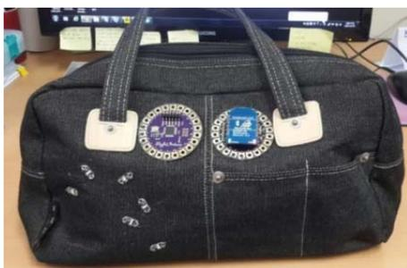
Fig.3. LilyPadArduino application using bluetooth
