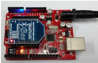
Fig.2. Arduino with Bluetooth module (FriBee)
