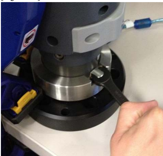
Fig.3. Installation FARO ARM
