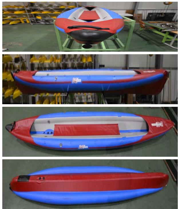
Figure 5: V-hull Kayak (Type 3)
