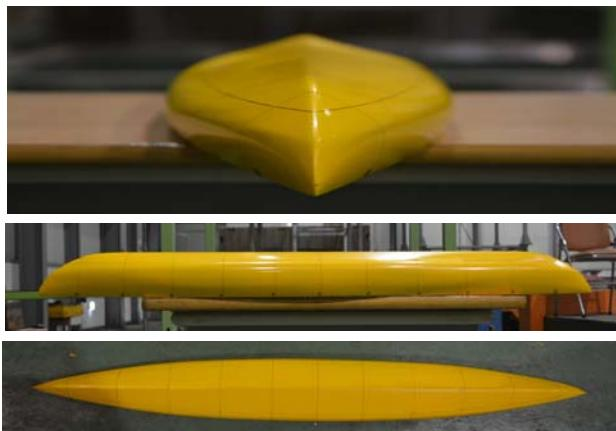
**Figure 11:** The reduced scale model ship (frame kayak, Type 1)
