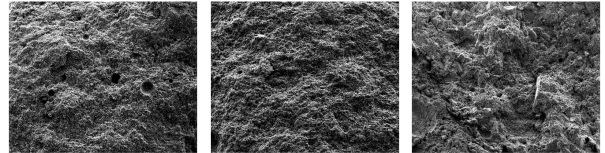
(a) Electron image of Portland cement specimen (b) Electron image of specimen adding Hardening agent (c) Electron image of specimen adding Feldspar powder & Hardening agent
