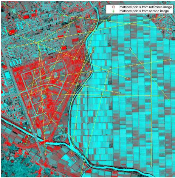
Figure 4. Matching points extraction by SURF method in site 1.
