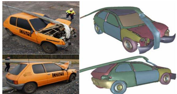
Fig. 1 Example of Crash Model by using LS-DYNA Program
