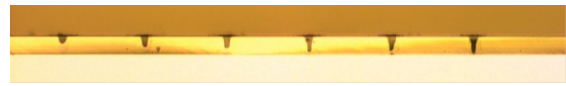
Fig. 3 A 50 \mu\text{m} thick glass substrate drilled with successively more pulses from a CO laser demonstrates the ability of this source to drill glass interposers, as well drill micro dots on light guide panels (LGP) used in display backlights. CO 2 drilling of this material typically results in heat related cracking.
