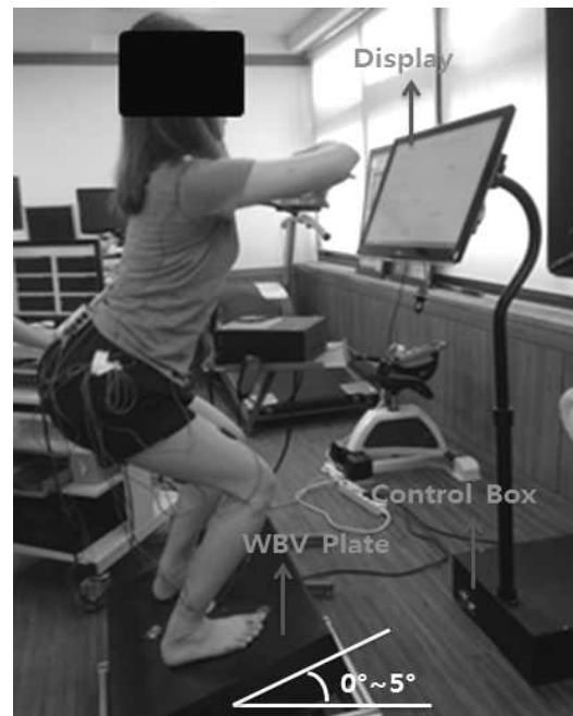
Figure 2. Squat exercise using Slope with vibration type of whole body vibration platform
