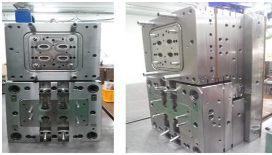
(a) 4 Cavity LSR-PBT MCM Mold
