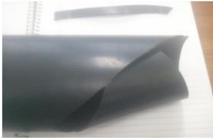
Fig. 2 Extraction of the specimen from the air bag for the tensile test
