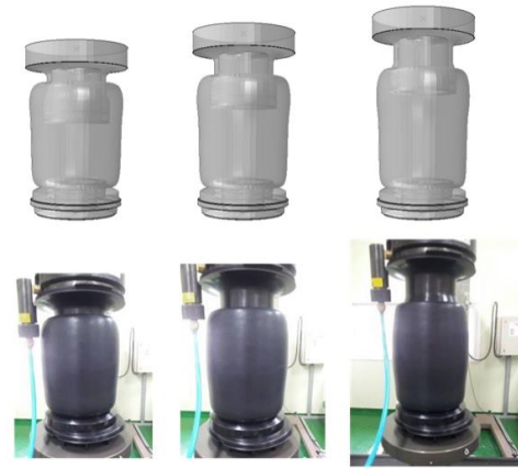
Fig.11 Comparisons of deformed shapes (bump, design height and rebound) between the simulation and the experiment
