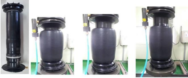
Fig. 1 Static experiments of an air spring for automotive at the unmounted, the bump height, the design height, and the rebound height
