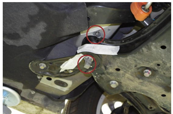
Fig. 6 Experimental setup to calculate the excitation force acting on bush using dynamic stiffness method
