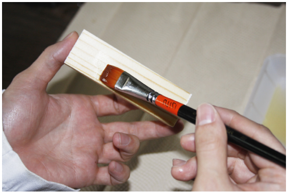
Figure 4. Appearance of the oil coating(Experiment in the transverse direction).
